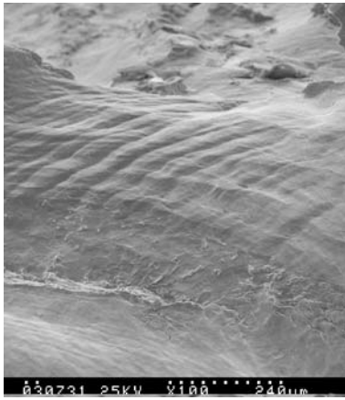
Figure 11 Secondary slip lines near the notch of 100Sn specimen strained to 7.8% at 298 K (high displacement rate, \dot{L} = 1 \text{ mm min}^{-1} , load direction in horizontal).
